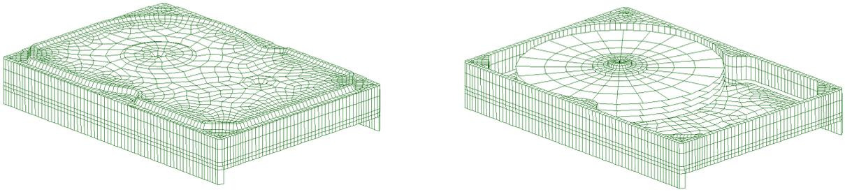
**Fig. 3:** Finite/boundary element mesh of detailed model (right-hand side without top cover)
