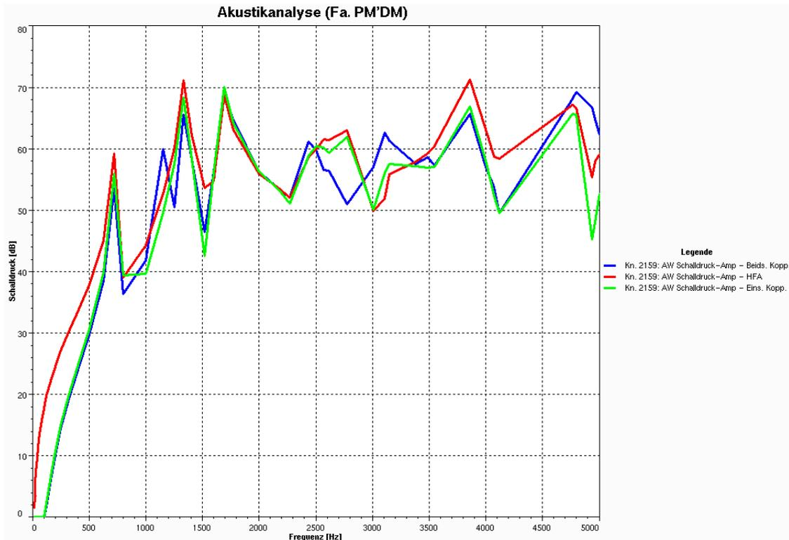
**Fig. 2:** Sound pressure level over frequency for different acoustic analysis types
