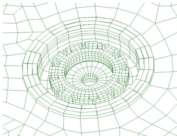
**Fig. 7:** Refined mesh of stator
