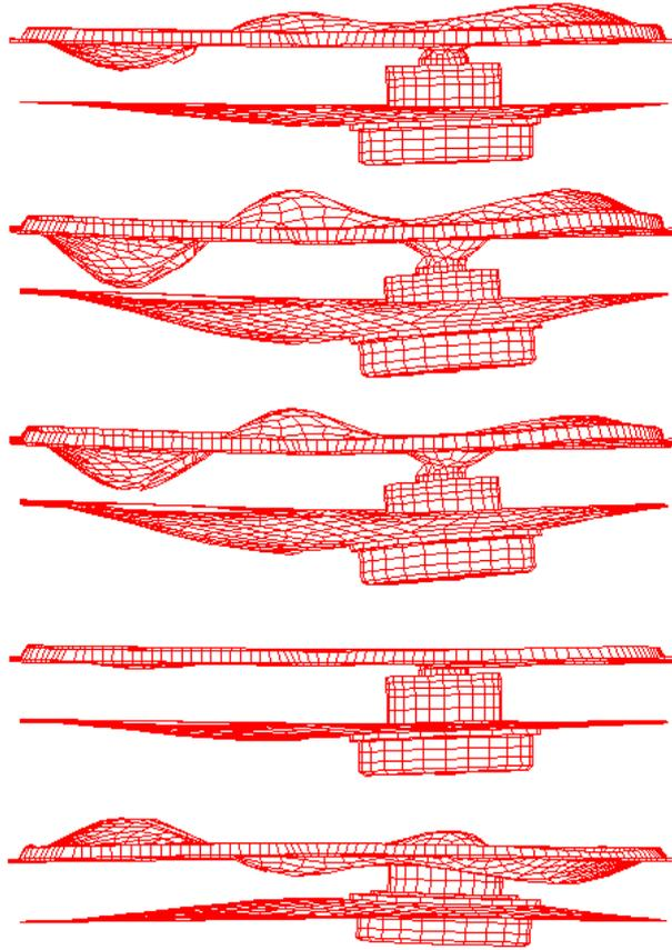
**Fig. 6:** Displacements of housing at a frequency of 2150Hz for phase angles 0, 45, 90, 125 and 180 degrees (from top to bottom) for pure radial excitation
