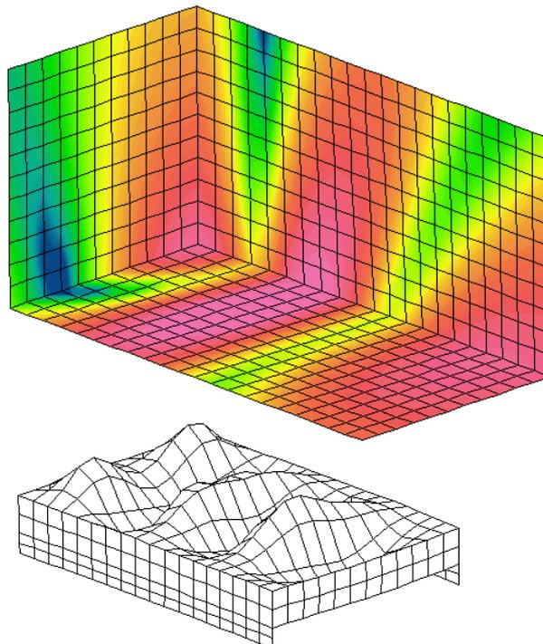
**Fig. 1:** Typical sound pressure level distribution for simple model
