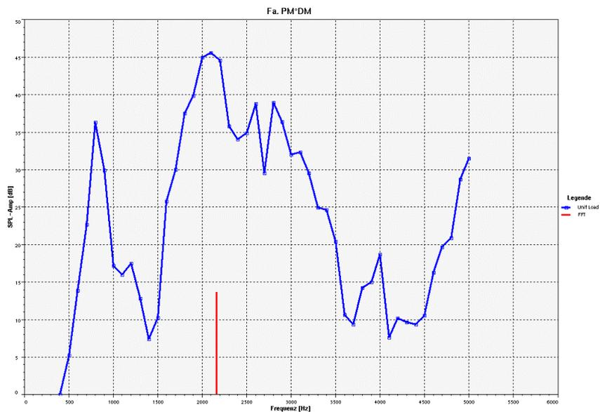
**Fig. 5:** Distribution of sound pressure level at reference point due to FFT and unit load
