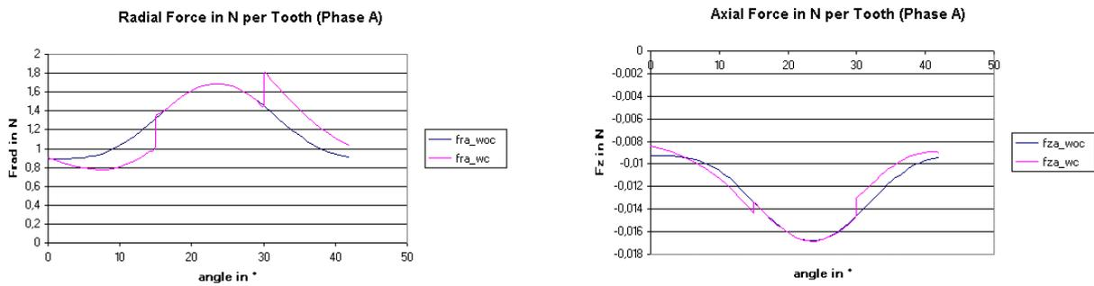
**Fig. 8:** Radial (left) and axial (right) forces due to detailed electromagnetic analysis
