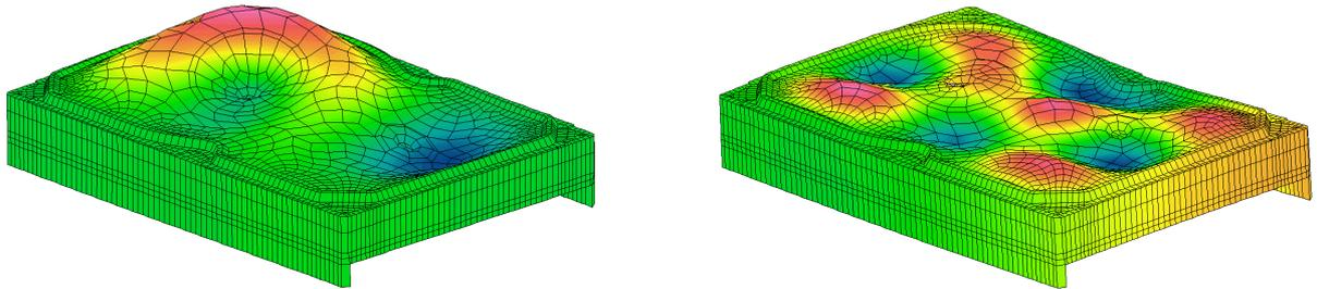
**Fig. 4:** Typical plot of vibrating housing for two different frequencies
