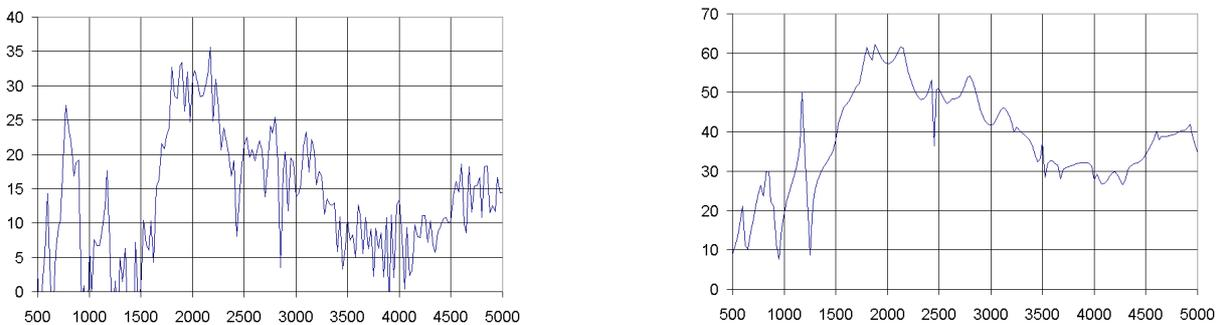
**Fig. 9:** Sound pressure level with axial/radial forces out-of-phase (left) and in-phase (right)
