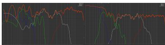
Figure 4. Raw (left) and tuned (right) virtual frequency response
