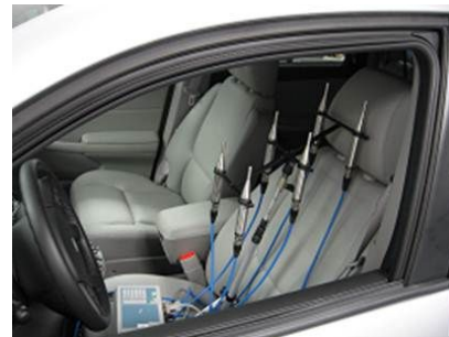
Figure 3. Typical measurement set-up for the localized sound power method
